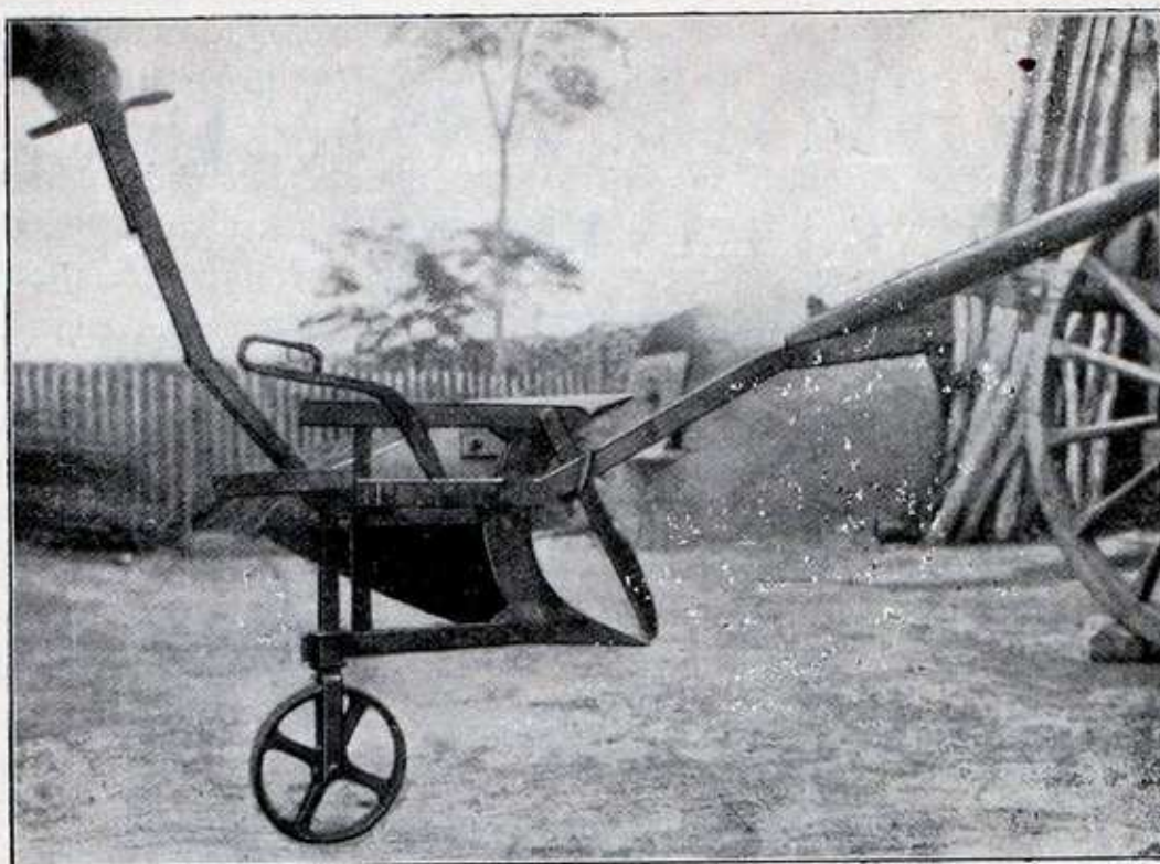
Plow with Double Mouldboard and Share.
